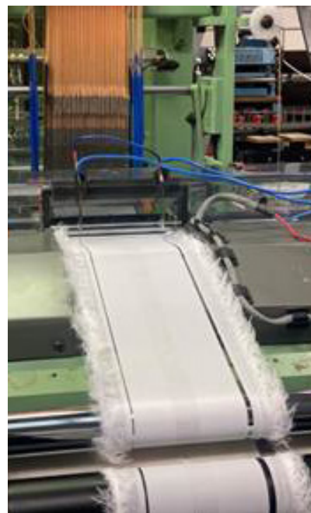
Fig. 4: Schematic illustration of the weaving process for textile sensors with long floating sections.
